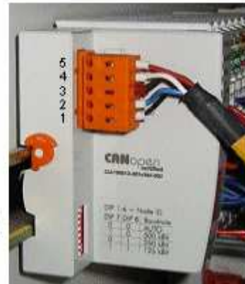
(Fig.3.3-9) PIN-OUT Conector CAN BUS
