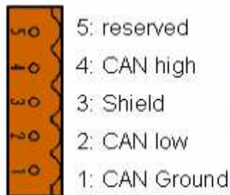
(Fig.3.3-9) PIN-OUT Conector CAN BUS
