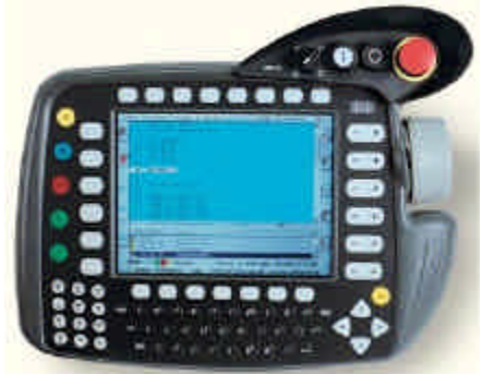
Figura 2.8 Panel de control KCP
