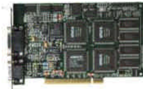
Figura 2.86 “Frame grabber” PC Vision de CORECO IMAGING
